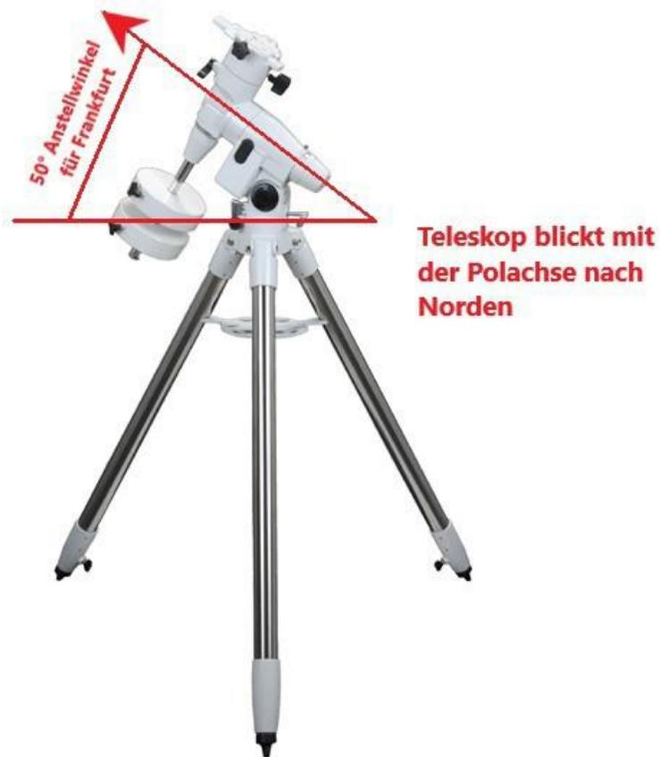
Since the earth rotates and the sky rotates from east to west, we can now easily track the celestial objects with the lower rotation axis of the mount. The more precisely you align the mount, the less you have to correct the tracking later with the upper rotation axis.
