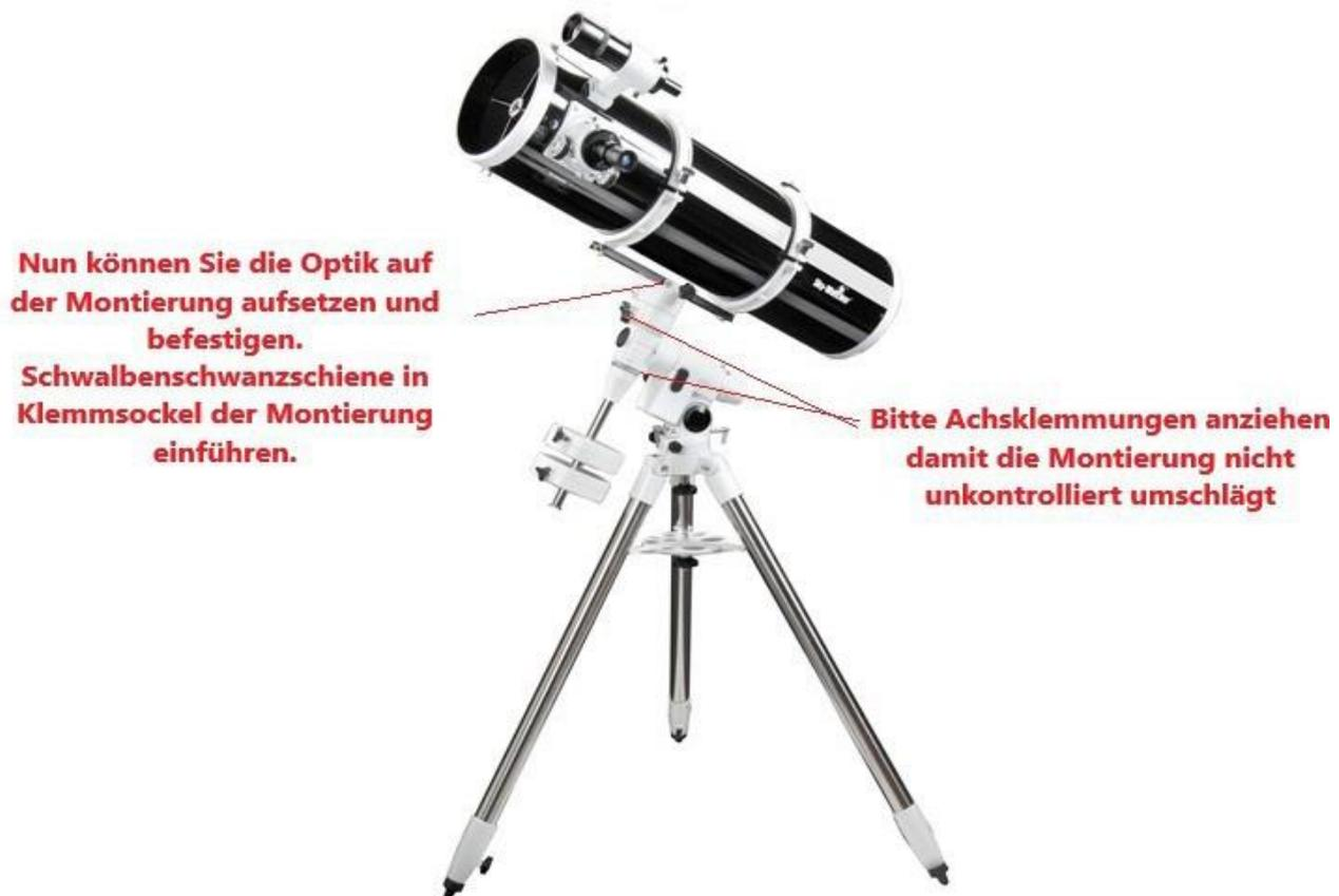
In order to use the system comfortably and safely, you must balance the weight of the optics on the mount. To do this, use the counterweights and prism rails/tube clamps as shown in the photos.
